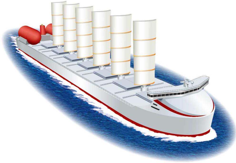
Figure Appendix 3.4-6: Bird's Eye View of the bulk carrier (Supper-efficient LNG-fueled Ship)
