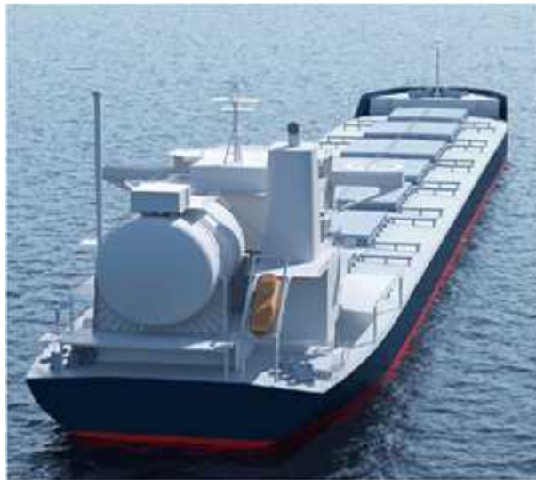
Figure Appendix 3.2-7: Bird's Eye View of the Ammonia-fueled 80,000 DWT Bulk Carrier (2)
